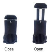
Your boat is equipped with a drain plug installed on the transom. When driving the boat, open the plug to drain the water on the floor. The water will automatically be drained by venturi effect. When launching the boat or stopping on the water, we recommend you keep the plug sealed. When the boat is lifted, stowed, stored, not used, or transported, drain plug shall remain open to drain any water that could fill the deck.
